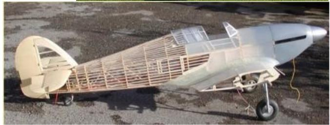
There are a few unusual features with this build such as the wings and front of the fuselage are skinned with 0.3mm thick fibreglass sheet and that the whole aircraft is made up from laser cut parts similar to current ARF practice
